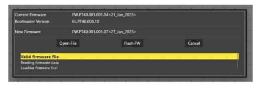
15) Once the Flash FW button is clicked, a pop-up will ask you Turn off the vehicle and remove the key from the ignition. If the ECU is connected to the vehicle, make sure to turn off the vehicle and disconnect the ECU from the vehicle. Once it is disconnected, Click on **YES** to proceed.
