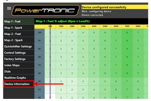
3) Observe the Bootloader Version and the Firmware version. (Make sure the Firmware version on the website is newer than the one in the ECU. If the Firmware on the website and on the ECU is the same, then no need to update the Firmware.)
