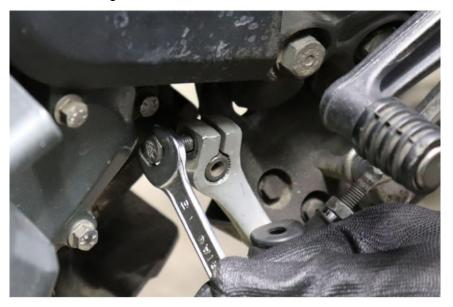
3) Install the supplied quickshifter, in the following order as shown in the image.
