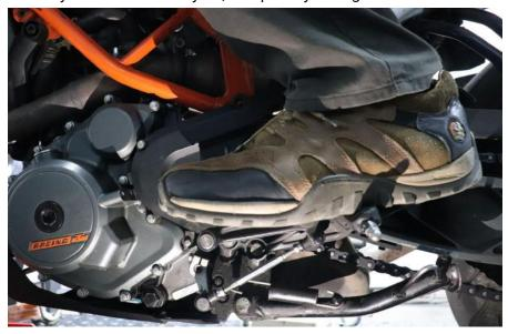
2.3. Move the shift lever like shifting up a gear, like going from 1st to 2nd, or 2nd to 3rd, etc.
