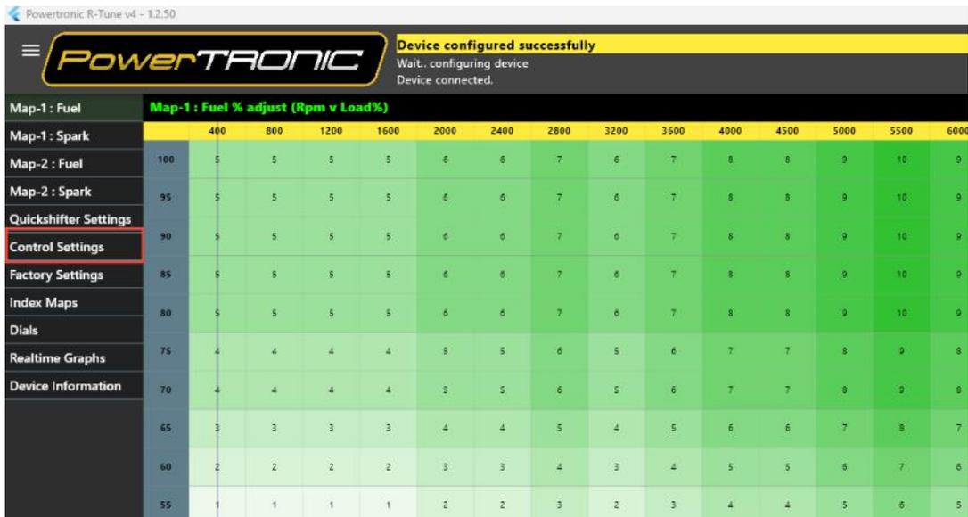
6. Select **Throttle Position/Injection Pulse Width** from the **Load Channel Input** from the drop-down.
