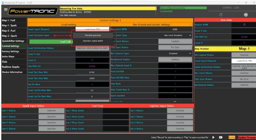
7. Click on **Load Calibration**. Follow the on-screen instructions in **Load Calibration Status**, Refer Figures below.
