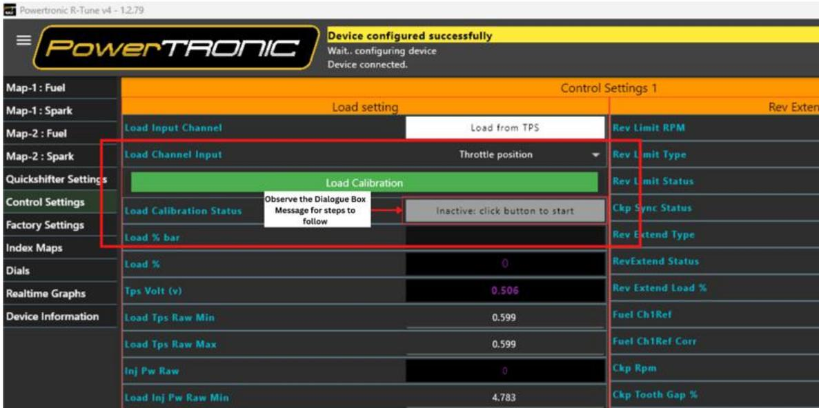
8. Click on **Load Calibration** and proceed as per the instruction displayed in the **Dialogue box** (This Step is recording the Zero Throttle Position)
