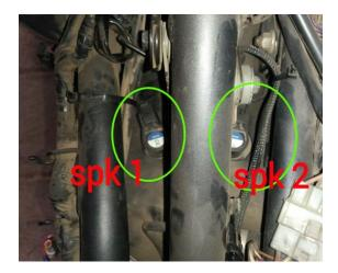
Step 5: Locate the TPS/CKP wires as shown.
