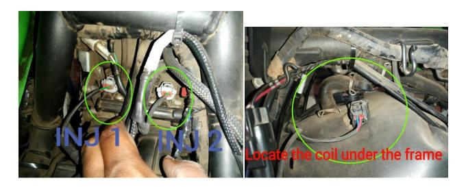
Step 4: Uncouple the stock injector/ignition connectors and connect the PowerTRONIC male and female wiring loom connectors.
