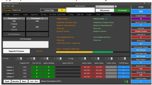
**Caution:** Upgrading the ECU would wipe all existing data on the ECU. Please make sure you have a fully charged battery or are connected to a power source in order uninterrupt the process.
