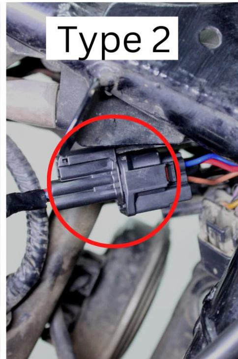
**4.1.15** Refer the **Image 18** to locate the Lambda sensor and Lambda Sensor Connector
