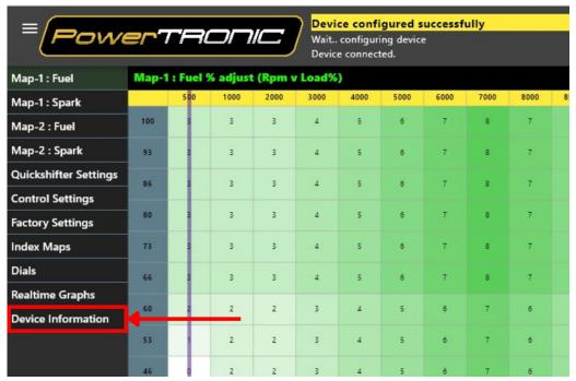
3) Observe the Bootloader Version and the Firmware version. (Make sure the Firmware version on the website is newer than the one in the ECU.)
