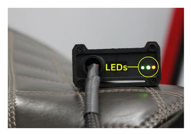
The blinking of the Red LED indicates that the Map on the FuelX is being activated. The Red LED starts blinking after the key and the kill switch are on.
