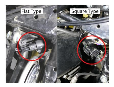
FuelX harness contains square or flat-type connectors depending on the model/year of manufacture/region. The customer can use the harness normally if the Lambda sensor connector and the FuelX harness connectors are matching by plugging in the male and female connectors.
