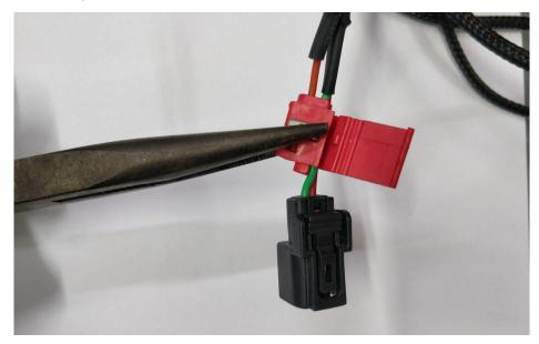
8. Once the metal clip goes in, lock the side of the tapping clip by pressing it, then lock the clip fully by attaching the cover.
