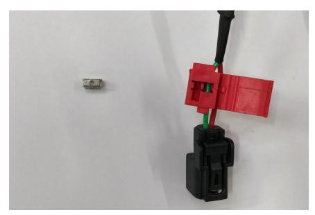
4. Please note in some cases, the customer has to cut and remove the sleeve that covers the wire to tap the wires properly.
