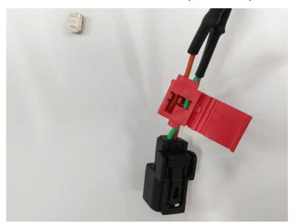
6. Insert the metal clip into the slot
